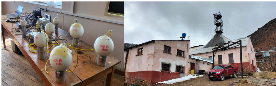
Figure 9: Bonner spheres of the SAMADHA spectrometer installed in Chacaltaya laboratory (left). The Chacaltaya laboratory in Bolivia (right).
