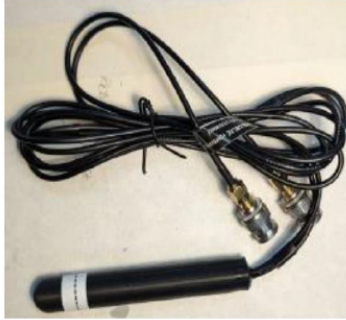
Figure 11: SiC+LiF and SiC-bare pair coaxially cabled and encapsulated in the 3D-printed, waterproof holder. Right: X-ray image of the detector complex.
