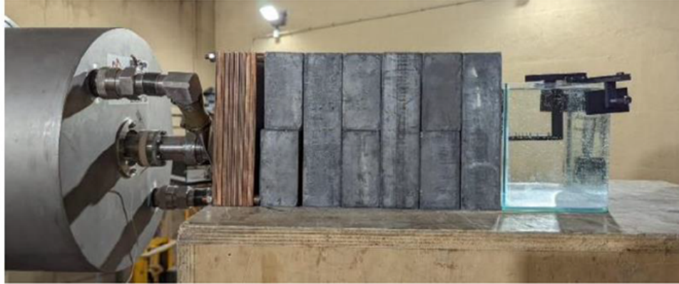
Figure 13: From left to right: FNG target, copper-lead energy degrader and water tank phantom embedding the 3D-printed activation foil holder.
