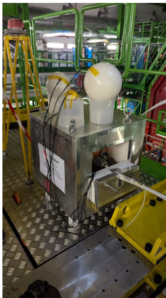
Figure 7: Experimental set-up in CMS cavern with 4 Bonner Spheres, each one containing a couple of SiCs (one bare and one covered with 6-Lithium Floride).
