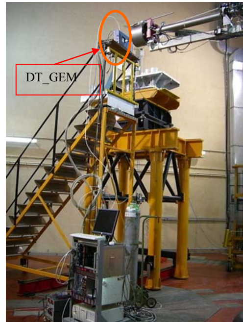
Figure 9 DT_GEM localized in front of the DT-neutron source at FNG (14.5 cm from the target).
