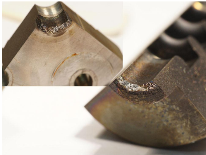
Fig 4 Highlight of molybdenum “extension tubes” failed adjacent to the SST flange in the left side of figure 2.
