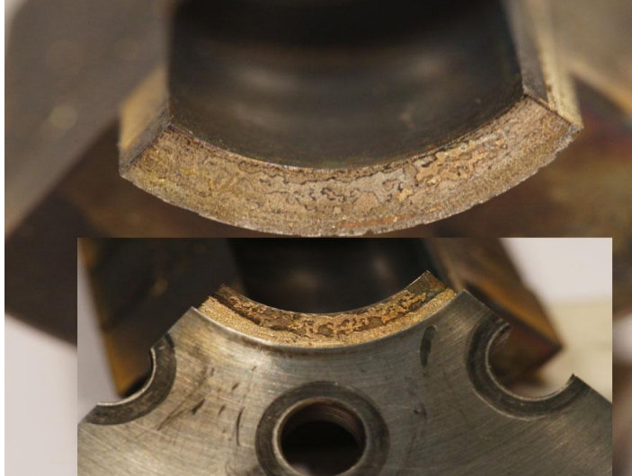
Fig 3 Highlight of joint failed in the right side of figure 2.
