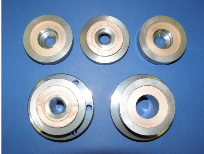
Fig 7 Components of moly structure, three cells plus connections to the end CF flanges
