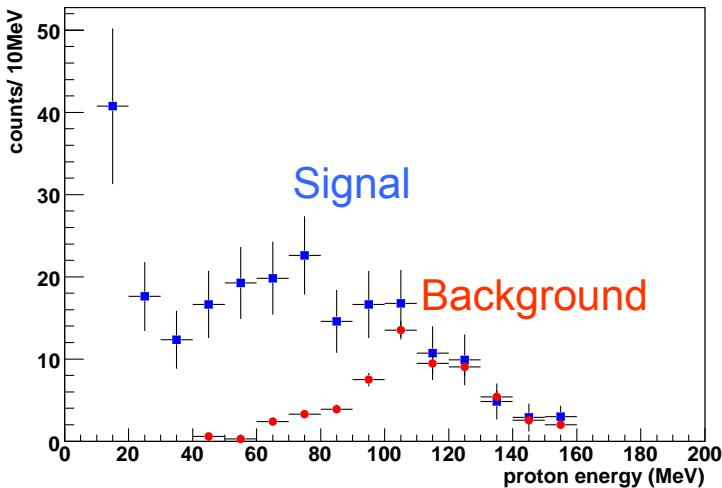
The background for the  ${}^5_{\Lambda}\text{He}$  has been evaluated taking with simulation of the K-np absorption reaction by subtracting the spectrum of the protons in coincidence with a  $\pi^-$  in the momentum region 267-272 MeV/c
