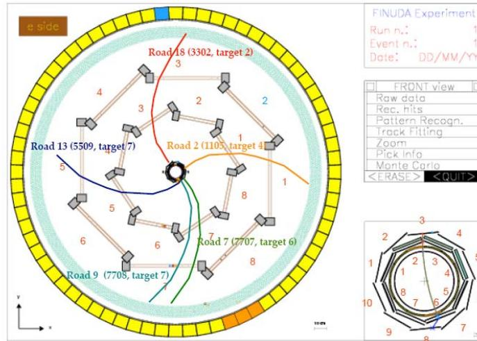
Figure 1.1: Typical layout of the FINUDA tracking region with a few examples of selectable “roads” for the study of detector subvolumes.
