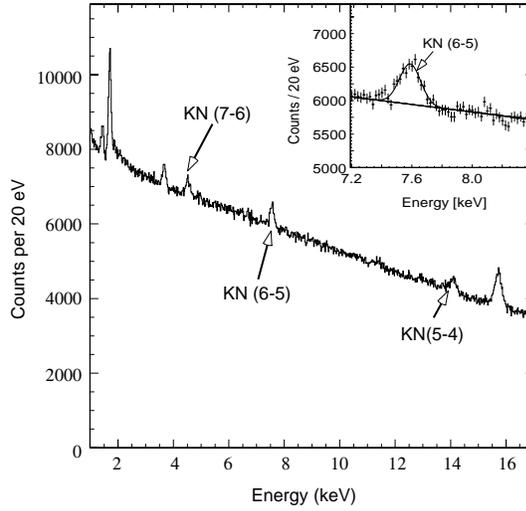
Figure 2: *Energy spectrum of kaonic nitrogen. The arrows indicate the position of the kaonic nitrogen X-ray lines. The peaks at 1.4, 1.7, 3.6 and 15.7 keV are the Al- $K\alpha$ , Si- $K\alpha$ , Ca- $K\alpha$ , and Zr- $K\alpha$  lines, respectively. The insert shows the fit of the  $6 \rightarrow 5$  kaonic nitrogen transition.*
