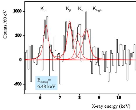
Figure 3: *Background subtracted kaonic hydrogen spectrum for an integrated luminosity of  $60 \text{ pb}^{-1}$ . Kaonic hydrogen lines  $K\alpha$ ,  $K\beta$  and  $K\gamma$  are fitted.*
