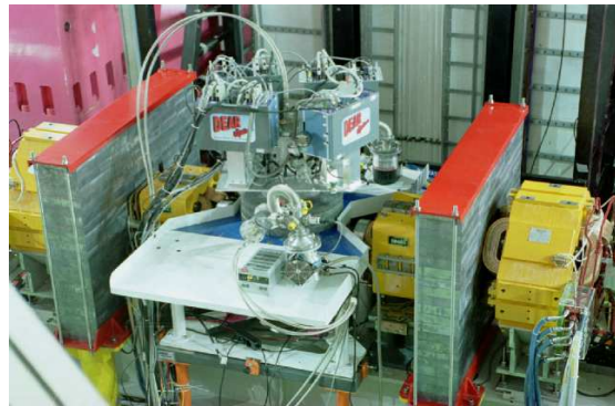
Fig. 3. DEAR apparatus installed at DAΦNE interaction point 2.
