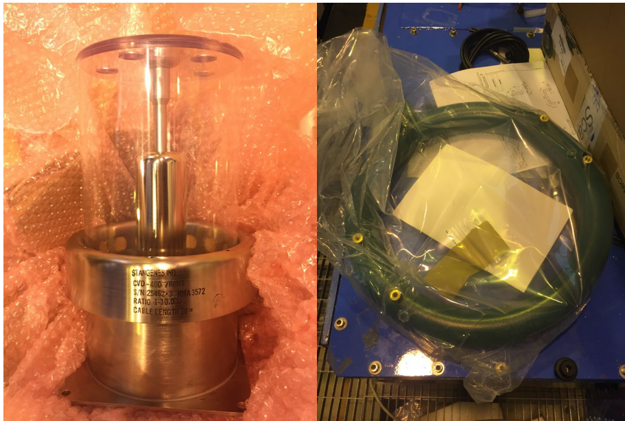
Figure 5: (Left) Capacitor Voltage Divider manufactured by Stangenes, (Right) Current Transformer manufactured by Pearson Electronics Inc.
