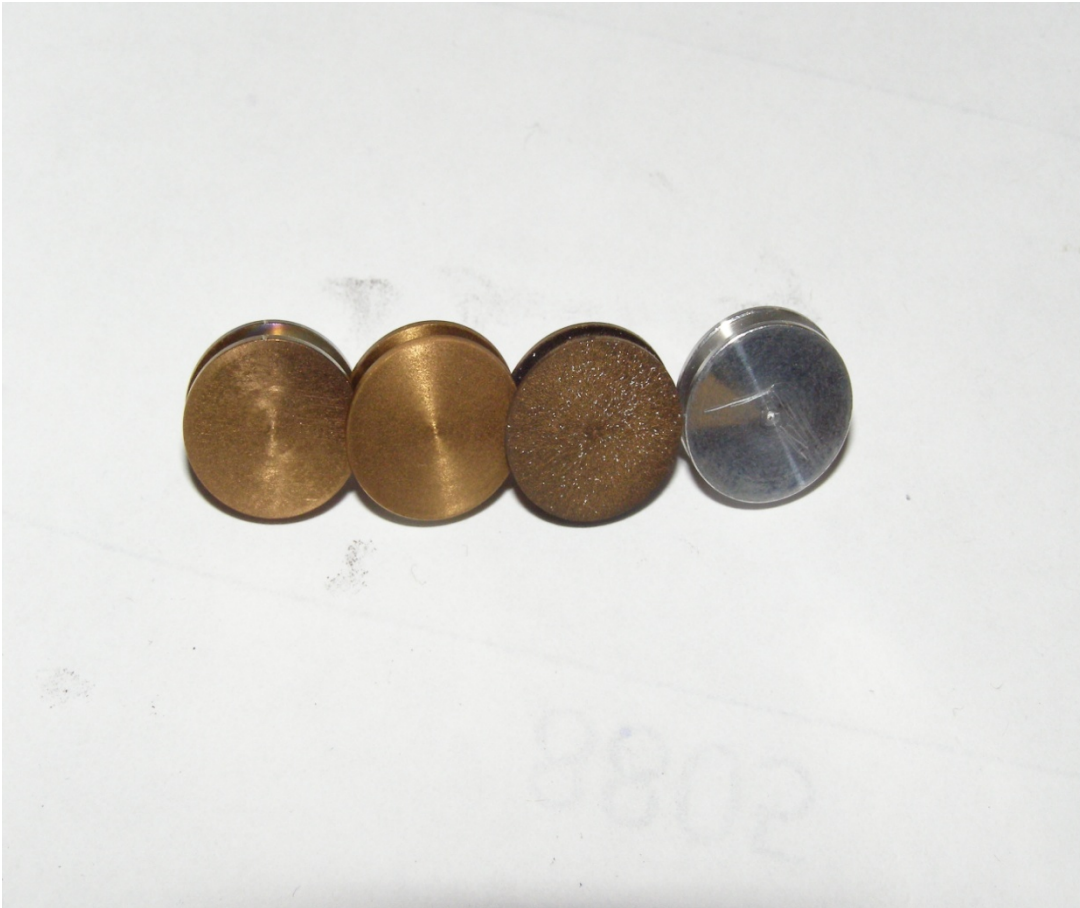
Fig 1 Aluminum samples covered by titanium nitride
